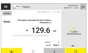
The DIDP control sample is incubated in parallel in the water bath and the initial and back weight of the aluminum foil disk measured. On the beaker the expected weight difference (control value) is printed and according to DIN EN ISO 75201 the measured value must not differ by more than  $\pm$  0.25 mg from the control value.
